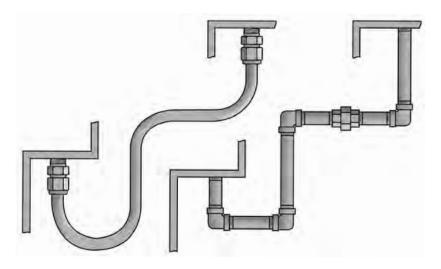
Whether it's a new construction or a retrofit, power plant tolerances can be tight. Swagelok offers small bore (up to 2 in. [50 mm] O.D.) tubing solutions to lessen the amount of installation space needed. Using tubing also improves safety by eliminating the need for welding in hazardous environments. And small bore tubing reduces the number of connections and potential leak points to improve fluid flow through the system. Learn more about Small Bore.
