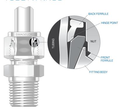
Want to know more about the Swagelok advantage? The special swaging action of our tube fittings helps you achieve a tight fit and reliable connection the first time, every time, to ensure fluid system performance. Learn more about Swagelok Tube Fittings.
