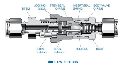
Simplify your installation even more—and still ensure fluid system integrity with Swagelok Quick-Connects. Push-to-lock connection means no tools or wrenching necessary. Learn more about our Quick-Connects.
