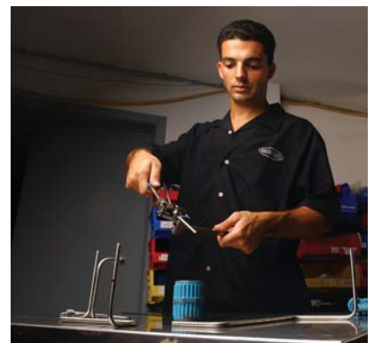
A Brownie's employee bends Swagelok tubing for use in a tankfill panel.
